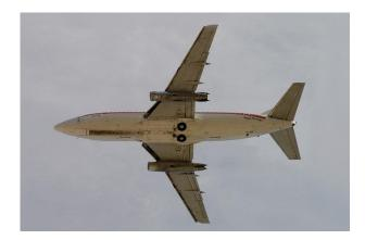
Above is the 737-200 produced in 1970. You can see that the two engines are almost directly under the two wings. In 1988, the production of 737-200 was ended after making 1,114 of planes of this model.
