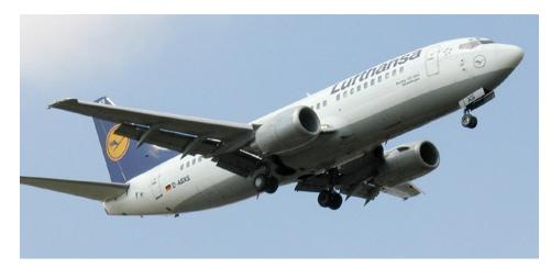
They also moved parts of the engine to the side of the fan. This gave the 737-300 engine the appearance of a hamster pouch. Here is a picture of the forward mounted hamster pouch engines:
