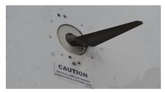
The AOA sensor is a small wing that can rotate and read the difference between the reference angle of the planes forward motion and the angle of the wind which is assumed to be the same as wind angle at the wing.
