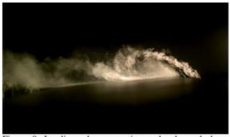
Figure 9: Leading edge separation and enhanced shear layer roll up, leading to the formation of a vortex. AoA = 10Deg, Ti=12.3. [18]
