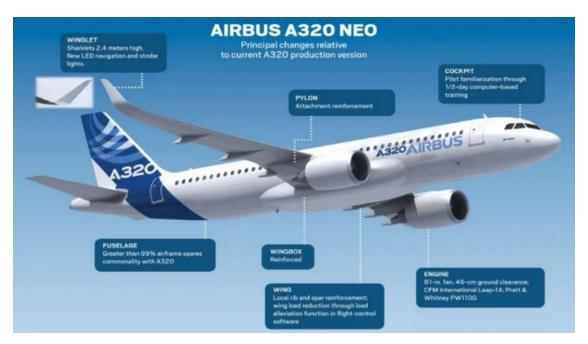
According to the following document, the A320-200 has 24 inches of clearance from the bottom of the engines to the ground and the A320-NEO has 18 inches of clearance. <u>https://www.airbus.com/content/dam/corporate-topics/publications/backgrounders/techdata/aircraft\_characteristics/Airbus-Commercial-Aircraft-AC-A320.pdf</u>
